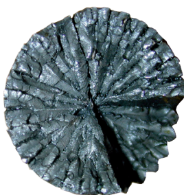
Alternate torsional fatigue
